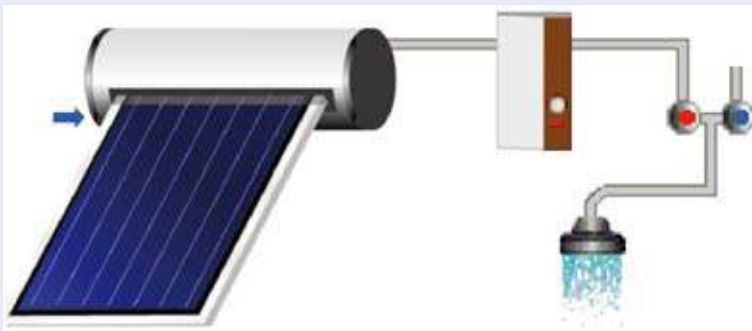
Figure 61: Hydraulic scheme of the domestic hot water thermosiphon reference system for single-family houses
