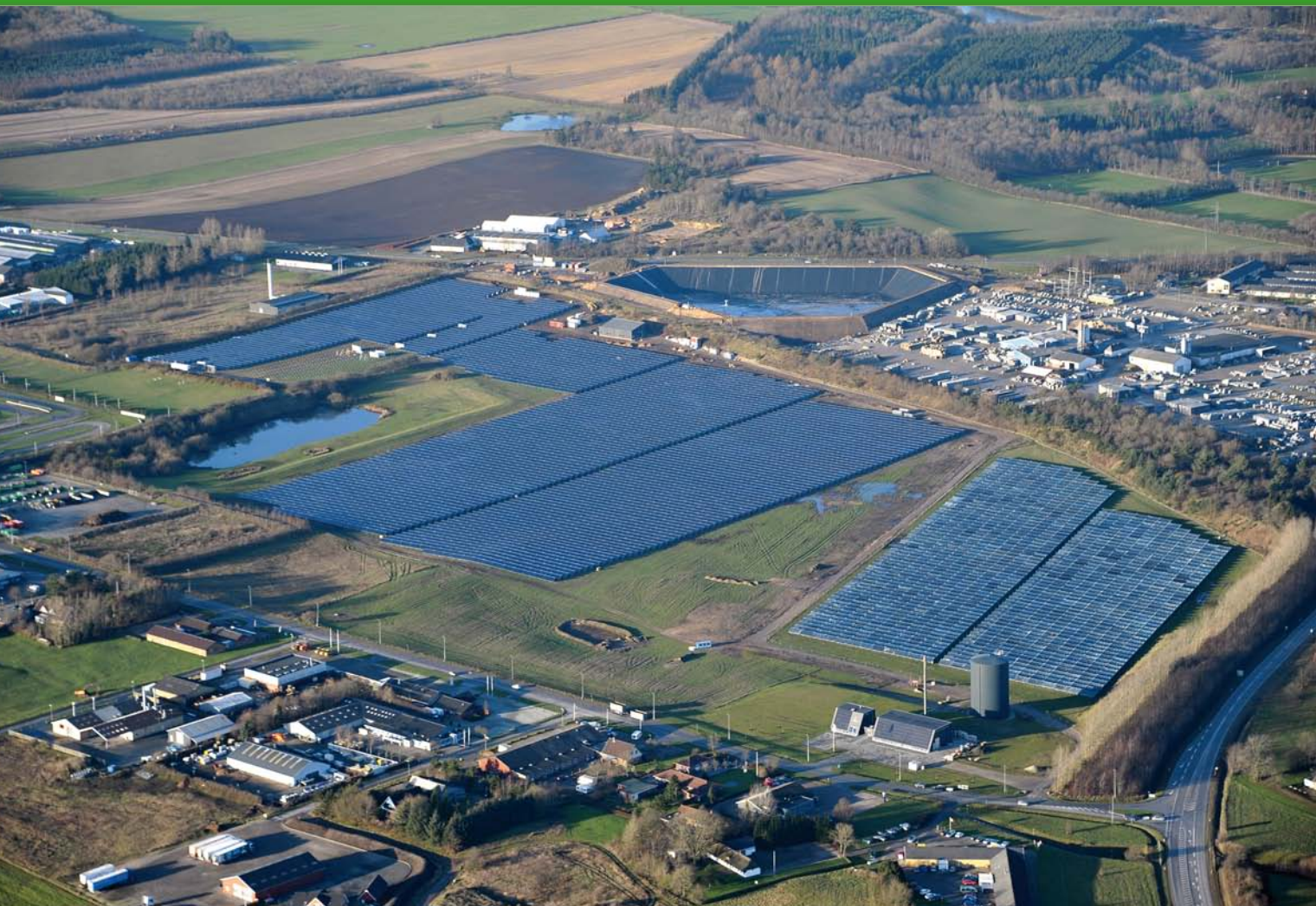
Solar district heating system in Vojens with load-balancing pit storage, Denmark.
