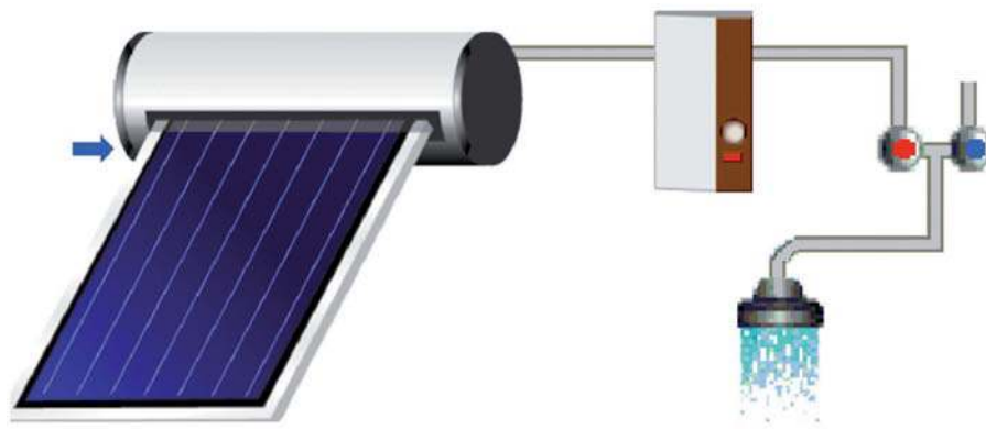
Figure 51: Hydraulic scheme of the domestic hot water thermosiphon reference system for single-family houses
